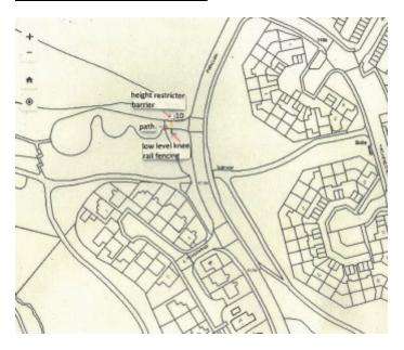
Height Restrictor Barrier: Supply and fit 1 2.10m (height to underside of arm) x approx. 5.00m wide height restrictor, as specified above.
