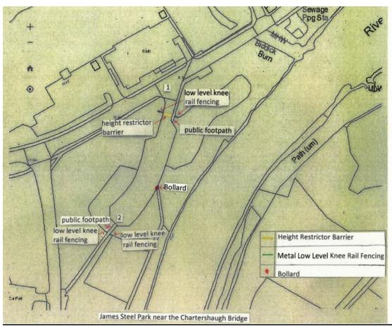
Height Restrictor Barrier: - Supply and fit 1 2.10m (height to underside of arm) x approx. 7.30m wide height restrictor barrier, as specified above.
