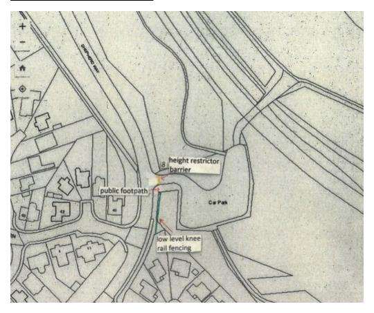
Height Restrictor Barrier: - Supply and fit 1 2.10m (height to underside of arm) x approx. 6.50m wide height restrictor barrier, as specified above.
