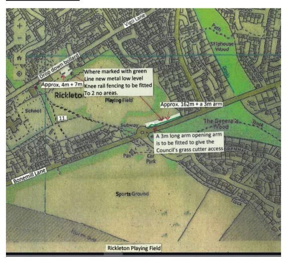
**Low Level Post and Rail Fencing**: To Bonemill Lane side supply and fit an approx. 162m long length of post and rail fence as specified above. Also supply and fit a 1 600mm high x 3.00m wide opening arm/rail into this fencing to match existing fencing with 2 posts and a shrouded locking area for customers own padlock next to drop kerb near the roundabout to allow the City of Sunderland Grass Cutter access onto the land.
