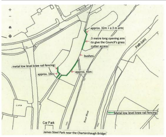
**Low Level Post and Rail Fencing**: Supply and fit 3 separate lengths of post and rail fencing as specified above . 1 length is to be approx. 32m long + an approx. 3m wide opening arm to match existing fencing is to be fitted into this length of fencing., Another length is to be approx. 45m long and the third length is to be approx. 19m long.
