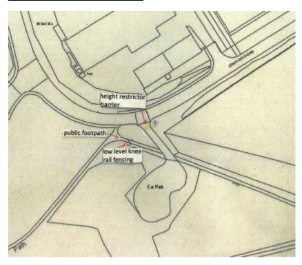
**Height Restrictor Barrier**: Supply and fit 1 2.10m (height to underside of arm) x approx. 5.50m wide height restrictor barrier, as specified above.
