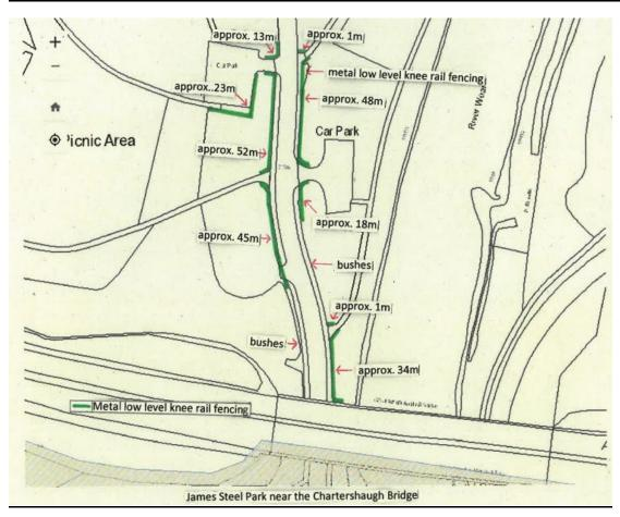
**Low level Post and Rail Fencing**: Supply and fit 9 separate lengths of low level post and rail fencing as specified above. The lengths are to be approx. 1m,48m, 18m,1m,,34m,45m,52m, 23m and 13m long lengths of fencing.
