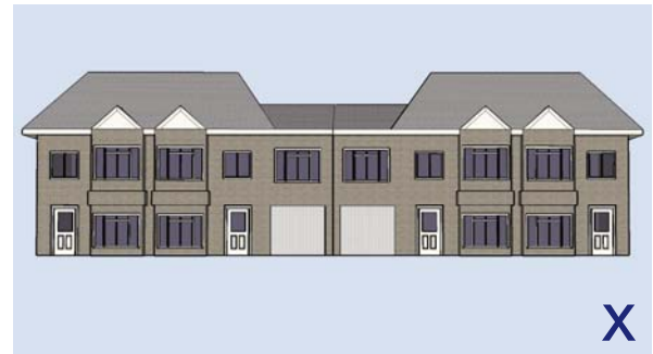
Side extensions that have resulted in the terracing effect.
